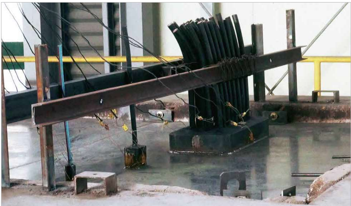
Image of Fire Test [A-60 class]
