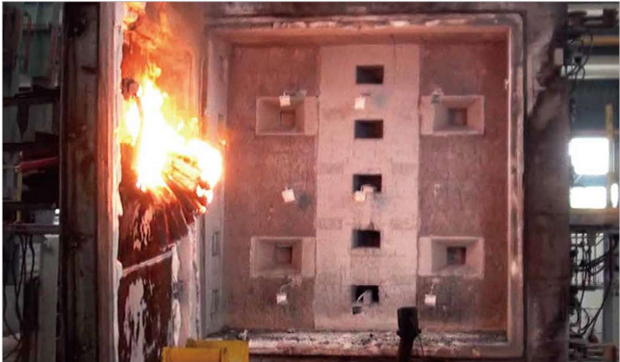
Image of Fire Test [H-120 class]
